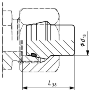
Figure 25 — Plug with O-ring (PL)
