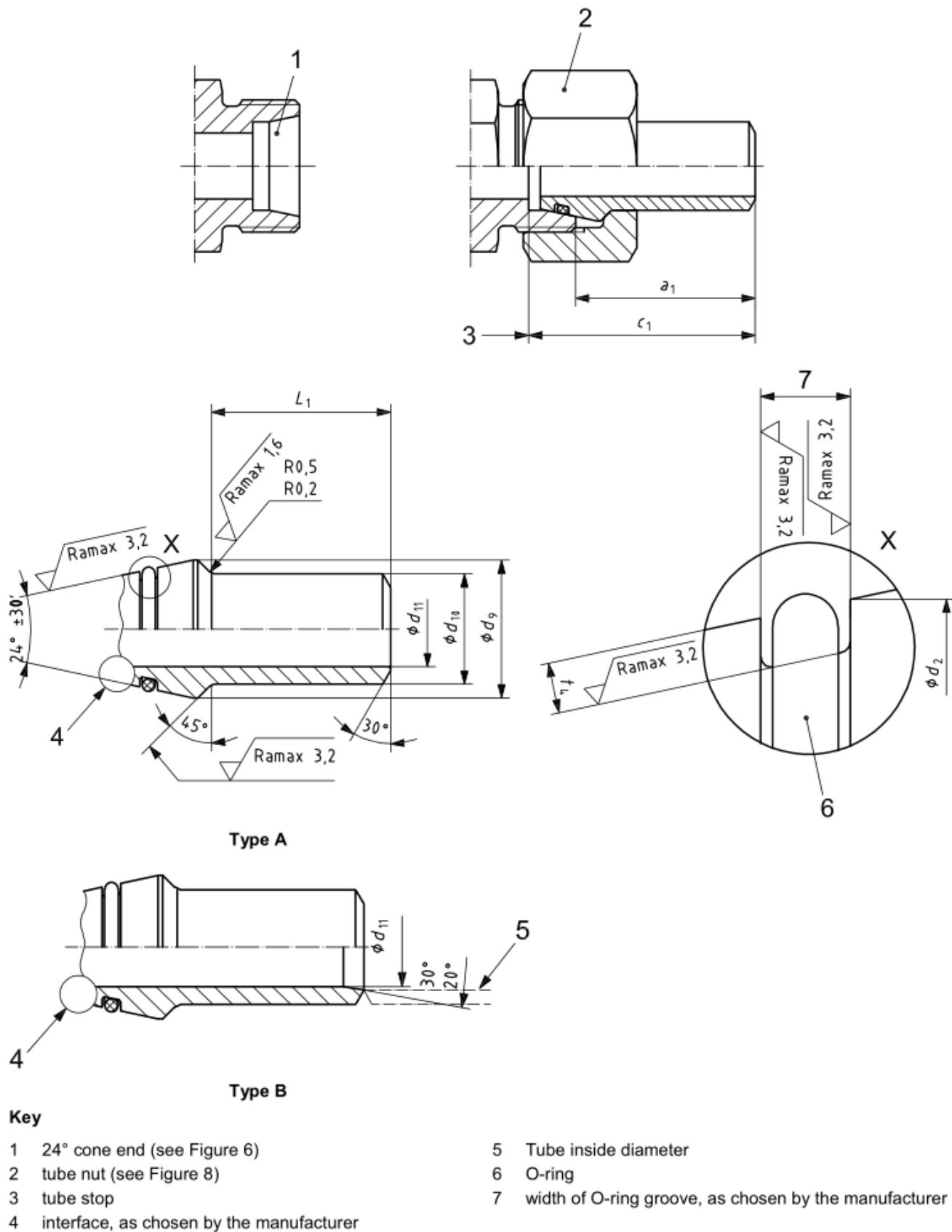
Figure 9 — Weld-on nipple (WDNP)
