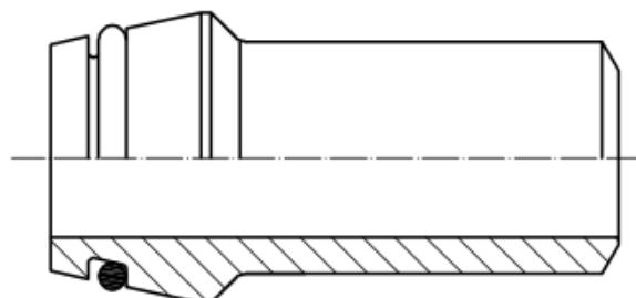
**Figure 5 — Weld-on nipple with O-ring (WDNP)**
