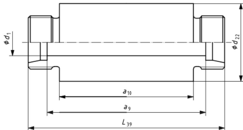
Figure 19 — Weld-in bulkhead straight connector (WDBHS)
