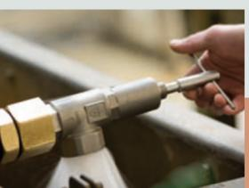
Pressure behaviour, throughput quantity and spring force are individually adjusted for each valve or fittings item. In the case of TÜV-certified components this setting is not to be changed afterwards. We naturally also supply fittings that the customer can adjust himself.
